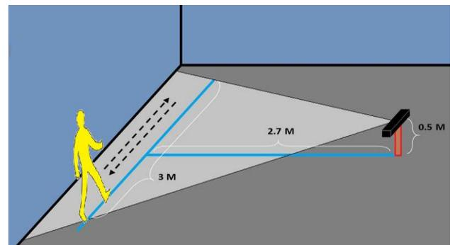
Figure 1: Kinect camera position with subject walking line.
